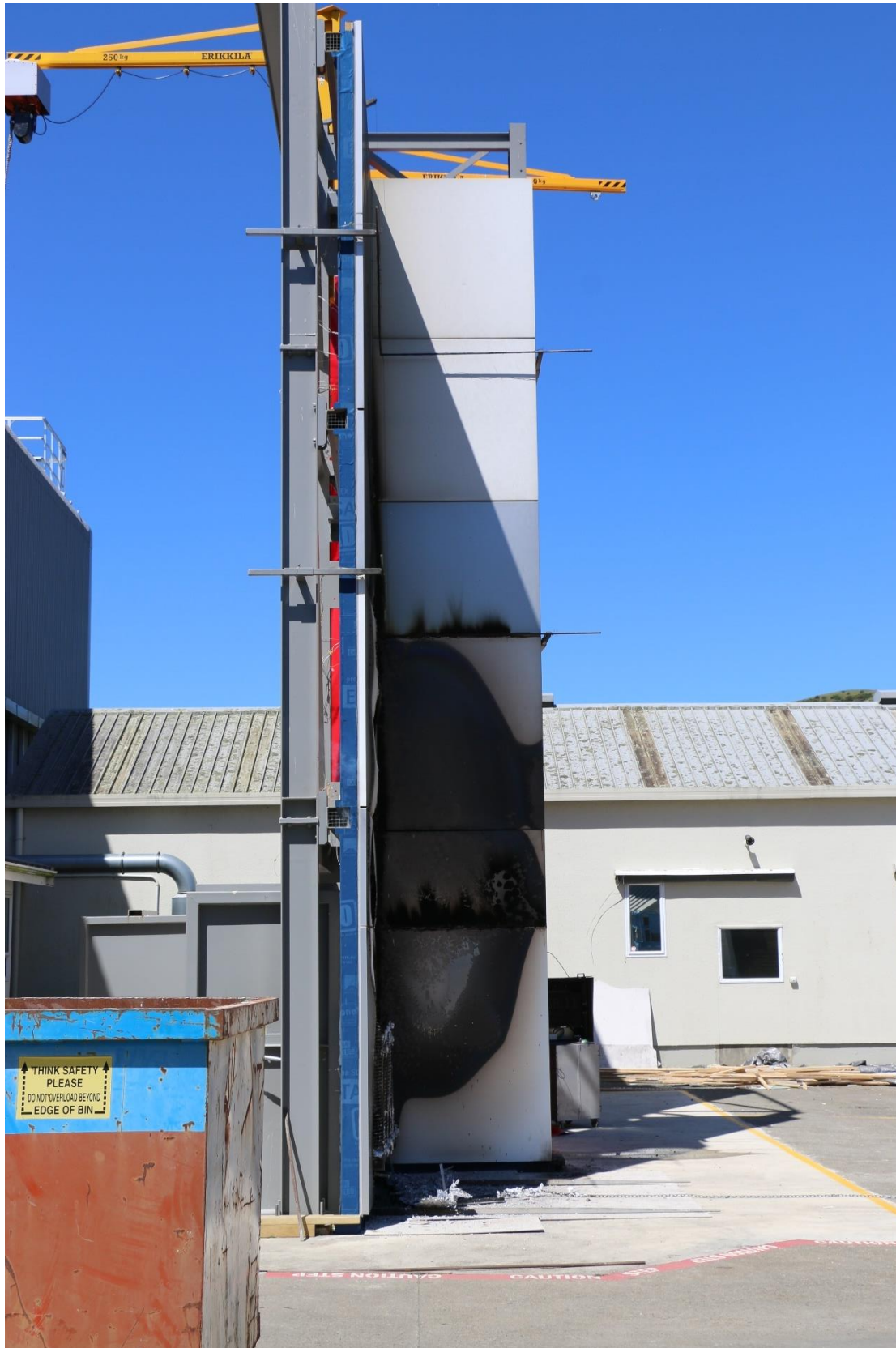
Photo 46: Post-test wing wall
