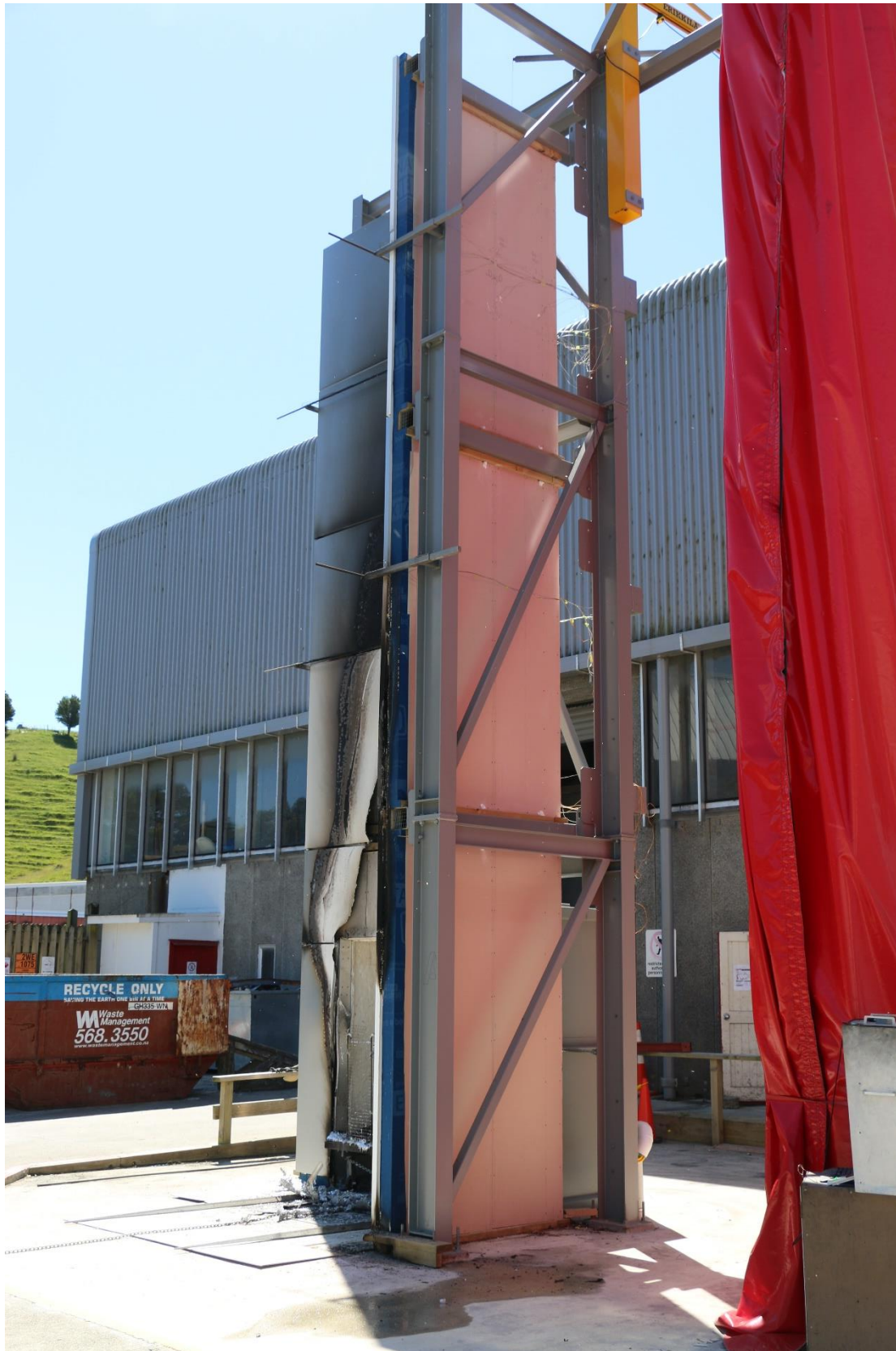
Photo 48: Post-test unexposed wing wall
