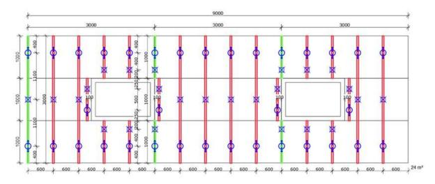
ALUCOBOND® – Panel with span 750mm – wall brackets and substructure:
