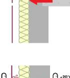
**Protection of the load-bearing wall:** The external thermal insulation protects from cracks due to temperature fluctuations. The cladding expands freely and avoids direct contact between the wall and climate change, thereby improving the durability of the building.
