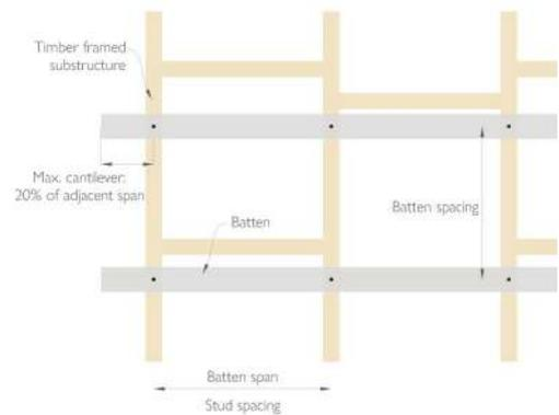
The following provides information in relation to the maximum span of the chamfered horizontal timber battens (maximum spacing between timber batten fixings connecting the batten to a timber stud frame, substructure) with respect to wind loading.
