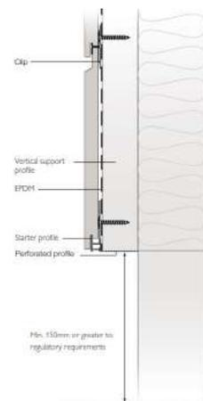
Schematic base detail (Refer to Cedral Construction Drawings for detailed drawings)
