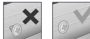
Use Cedral Click clip screw or rivet for fixing of the starter profile to support frame. Ensure the screw or rivet sits flush with the profile surface.
