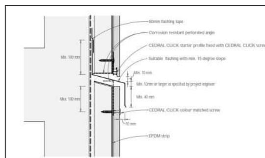
Example of horizontal control joint (inter storey) detail
