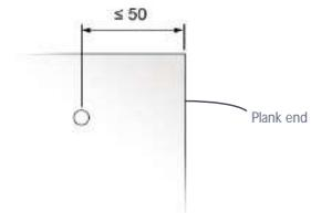
Predrilling required where Cedral metal screw falls within 50 mm from plank end
