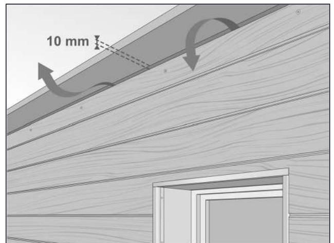
Min. 10 mm gap is required at the top of the façade for ventilation.
