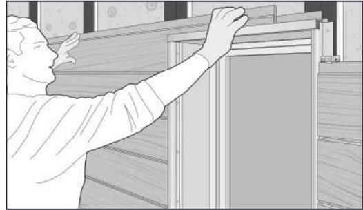
Allow minimum 10 mm gap at window/door head and sill interface for ventilation.
