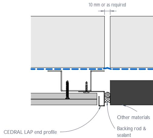
Figure 7: CEDRAL LAP vertical joint - Detail 2
