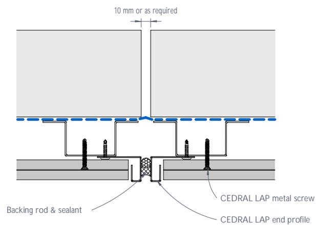
Figure 6: CEDRAL LAP vertical joint - Detail 1
