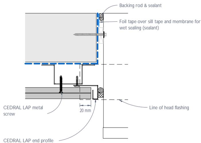
Figure 14: CEDRAL LAP meter box junction - Plan view
