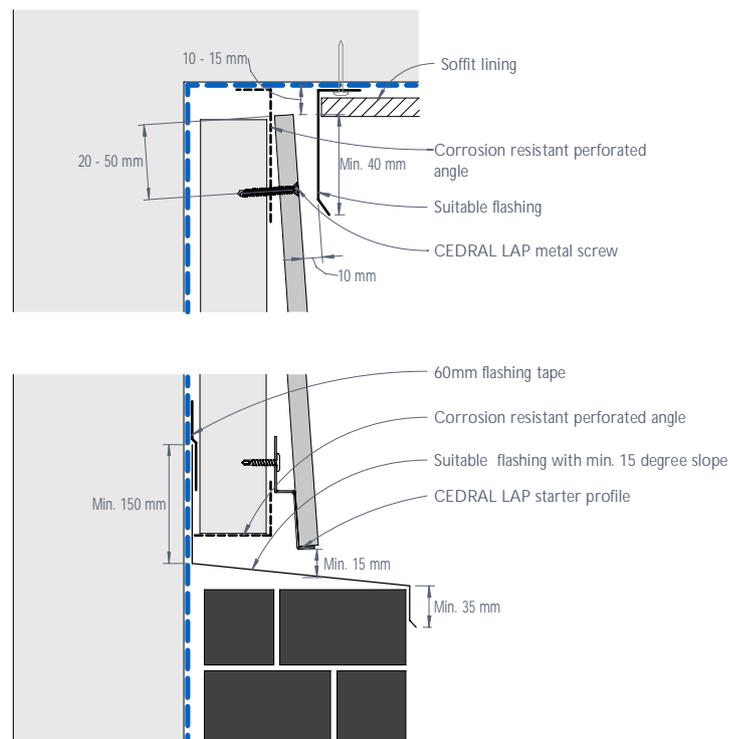
Figure 21: CEDRAL LAP junction with other materials, eaves or the like - Recessed detail
