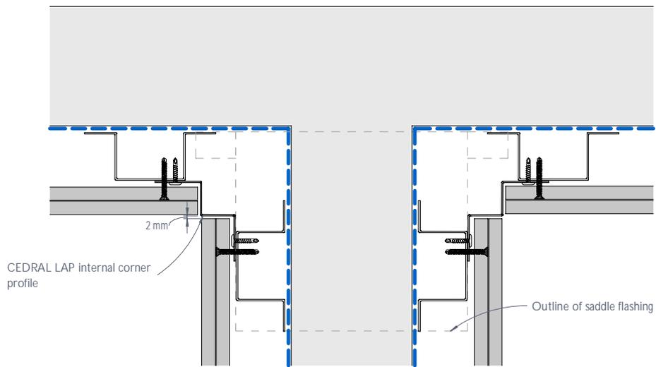
Figure 37: Parapet junction - Plan view
