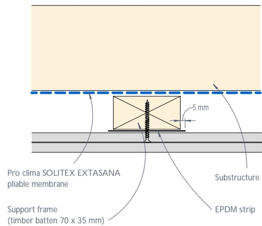
Figure 3: CEDRAL LAP Intermediate fixing detail - Plan view
