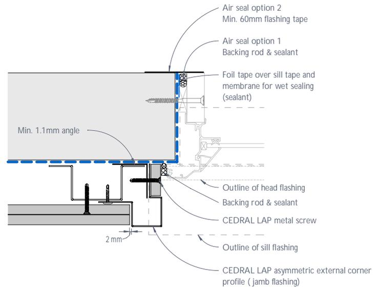
Figure 10: CEDRAL LAP window jamb junction or the like - Detail 1
