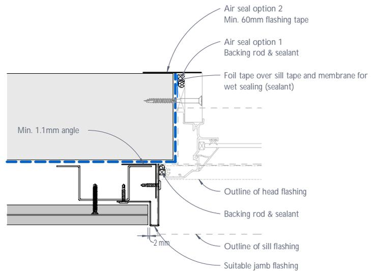
Figure 12: CEDRAL LAP window jamb junction or the like - Detail 3
