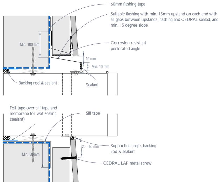
Figure 13: CEDRAL LAP meter box junction - Section
