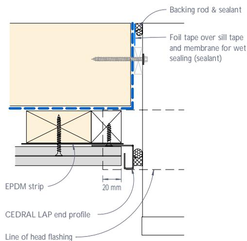
Figure 14: CEDRAL LAP meter box junction - Plan view
