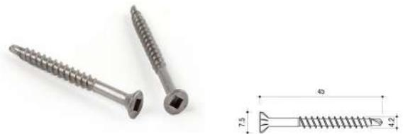
Cedral Lap colour matched mushroom head screw for fixing Cedral Lap to timber batten where fixings are visible
