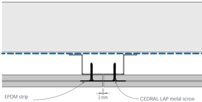
Figure 5: CEDRAL LAP Vertical joint - Plan view
