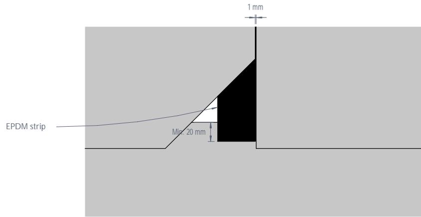
Figure 4: CEDRAL LAP vertical joint - Elevation
