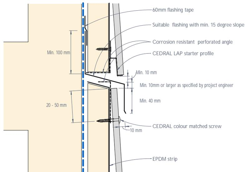
Figure 8: CEDRAL LAP horizontal control joint and inter-storey detail
