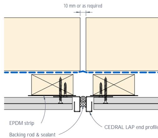
Figure 6: CEDRAL LAP vertical joint - Detail 1
