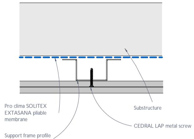
Figure 3: CEDRAL LAP Intermediate fixing detail - Plan view
