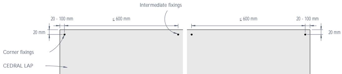
Figure 1: CEDRAL LAP fixings arrangement - Elevation
