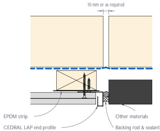
Figure 7: CEDRAL LAP vertical joint - Detail 2
