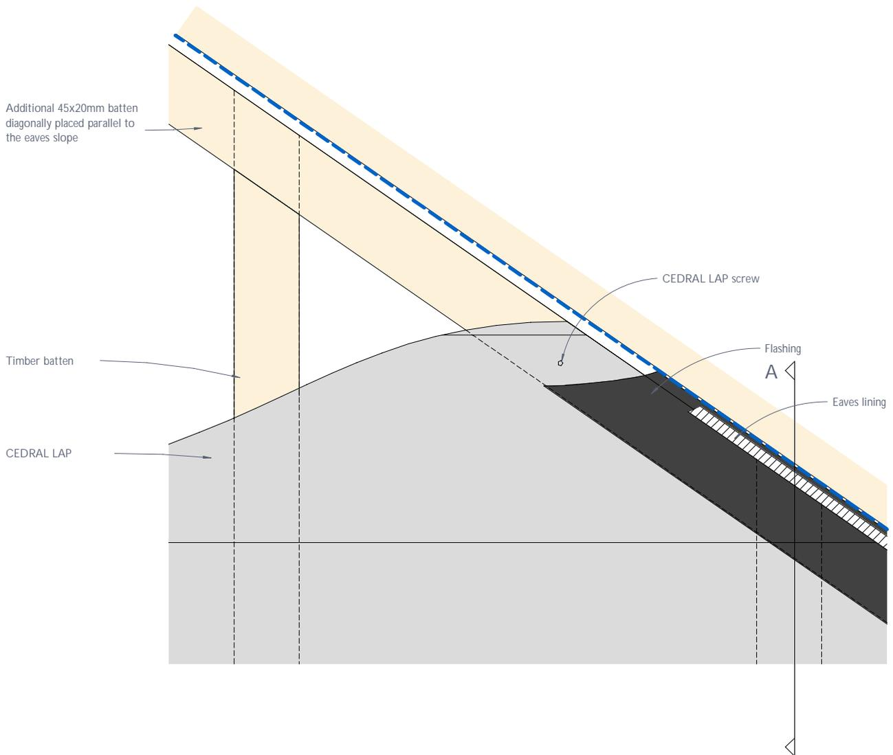
Figure 22: CEDRAL LAP junction with angled eave - Elevation
