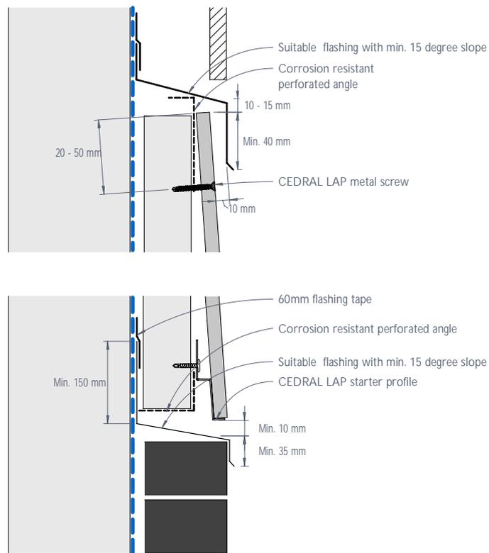
Figure 20: CEDRAL LAP junction with other materials - Flush detail
