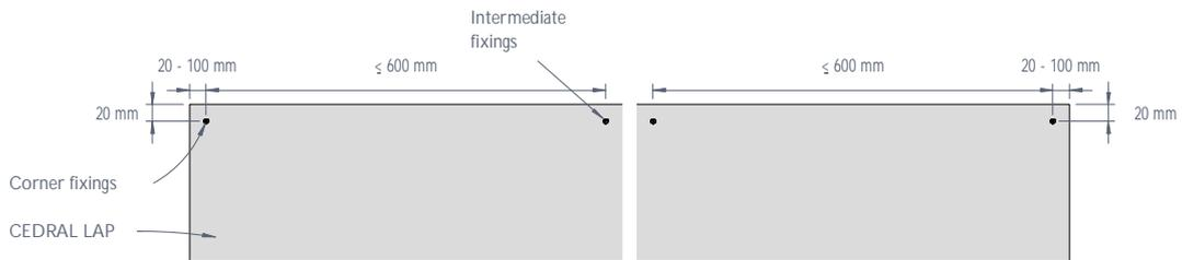
Figure 1: CEDRAL LAP fixings arrangement - Elevation
