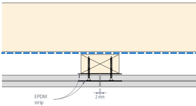
Figure 5: CEDRAL LAP Vertical joint - Plan view
