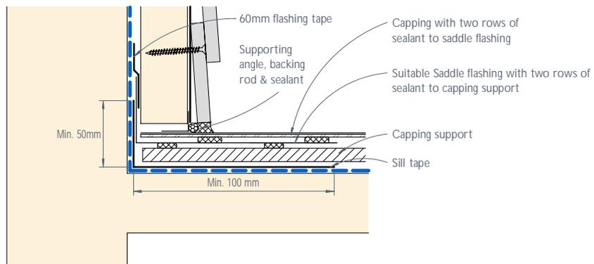
Figure 36: CEDRAL LAP parapet junction - Section
