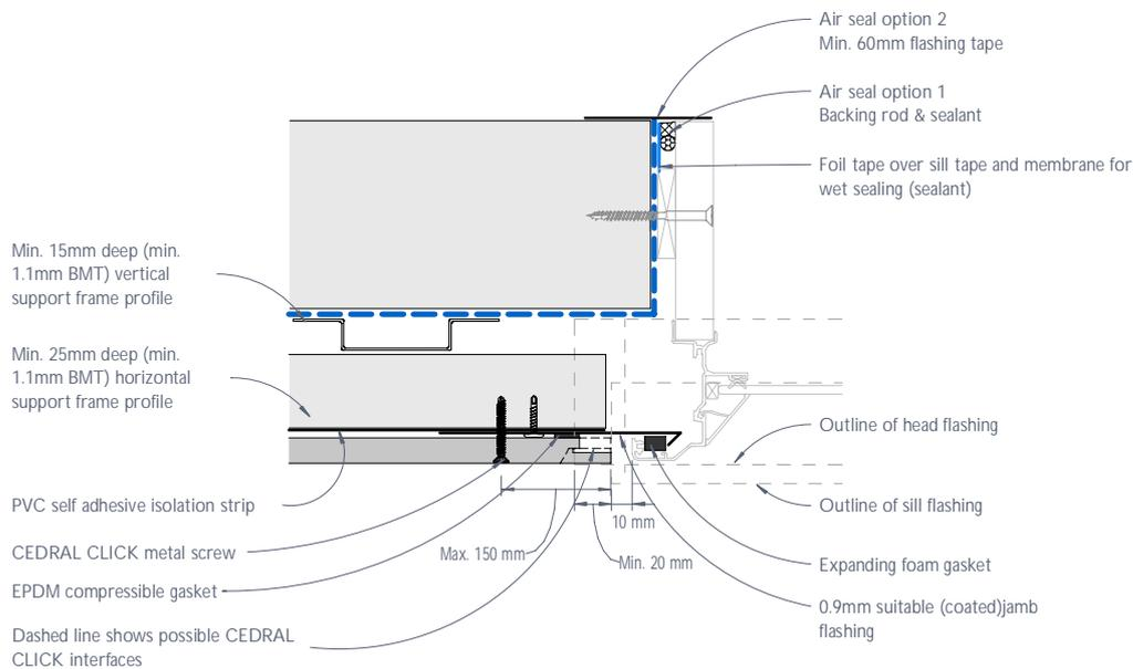
Figure 11: CEDRAL CLICK window jamb junction or the like - Flush detail
