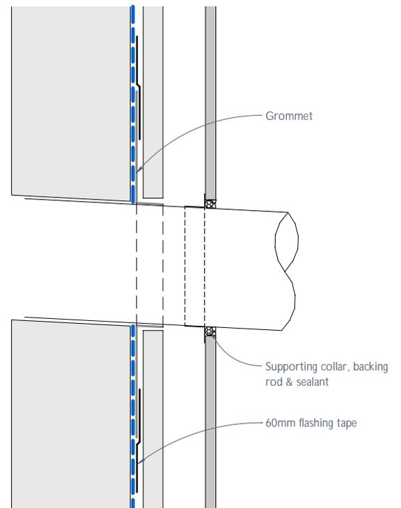
Figure 30: Pipe penetration - Section
