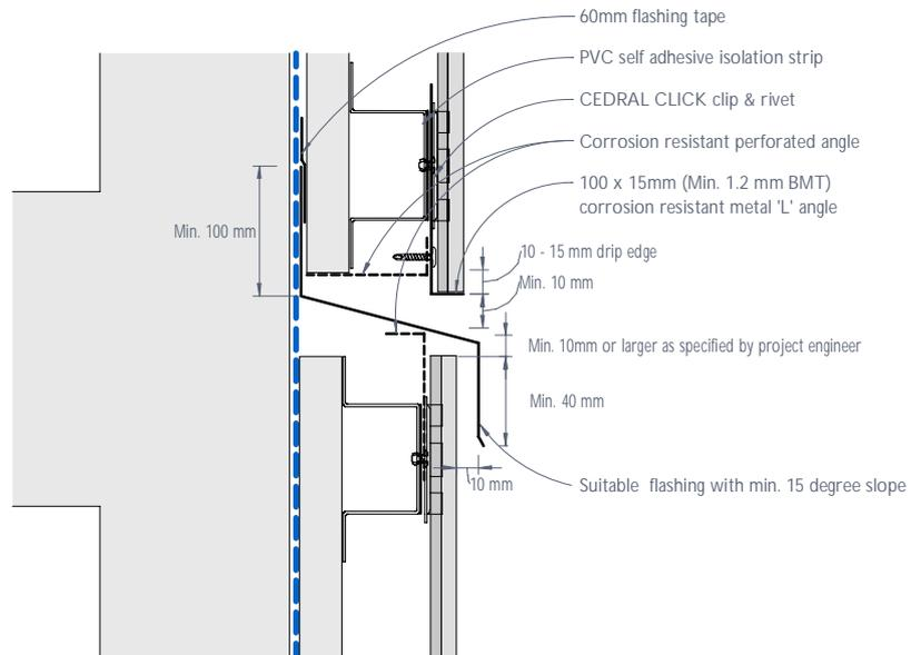
Figure 7: CEDRAL CLICK horizontal control joint and inter-storey detail
