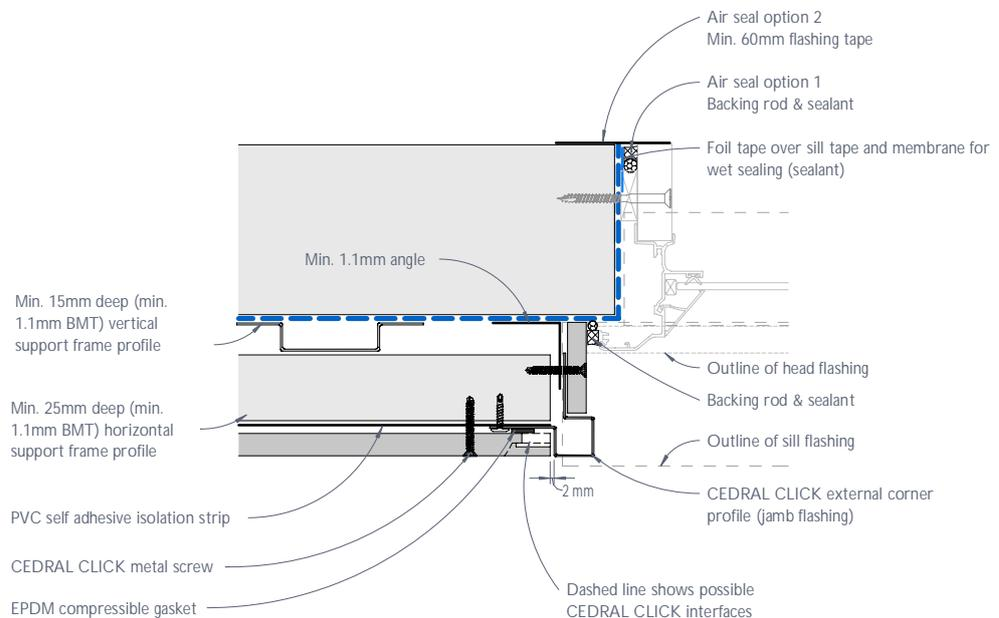
Figure 9: CEDRAL CLICK window jamb junction or the like - Recessed detail
