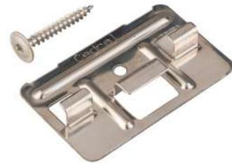
Cedral Click colour matched mushroom head screw for fixing Cedral Click to timber batten where fixings are visible (4.8 x 38 mm, head diameter ~12 mm, TORX T20, stainless steel 304)
