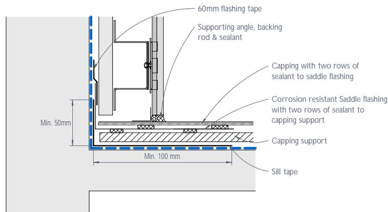
Figure 33: CEDRAL CLICK parapet junction - Section
