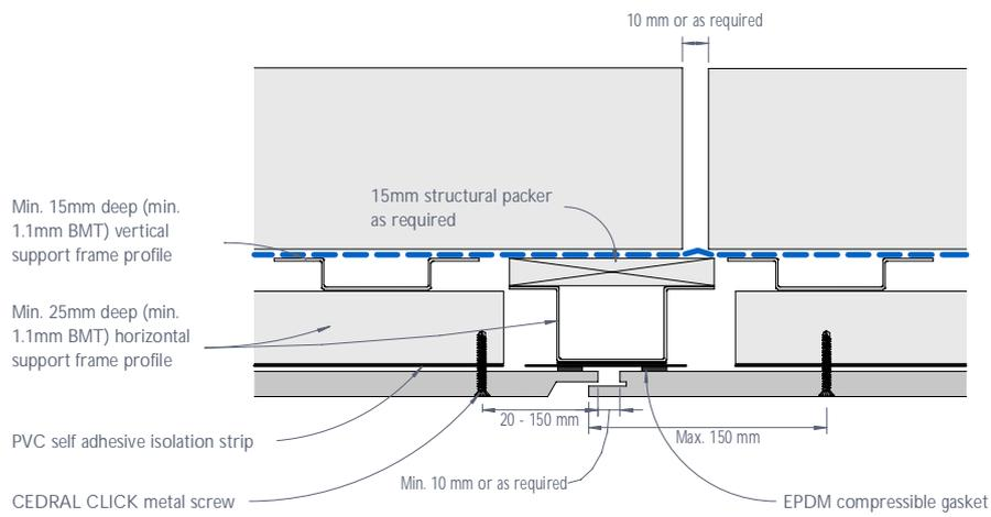
Figure 4: CEDRAL CLICK vertical control joint - Detail 1
