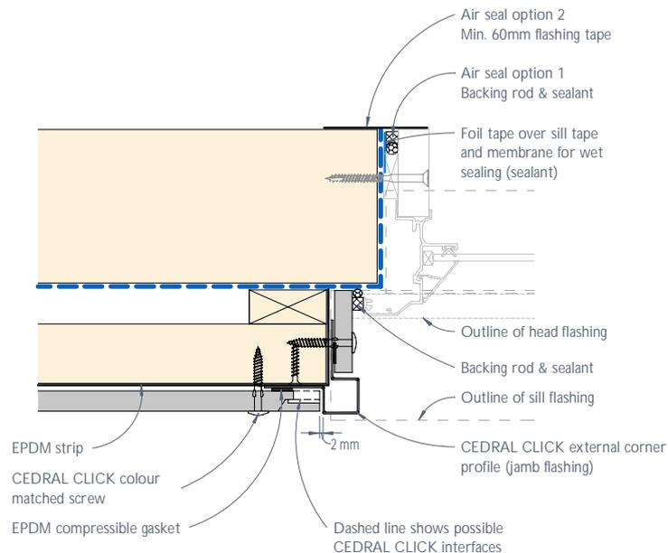
Figure 10: CEDRAL CLICK window jamb junction or the like - Recessed detail
