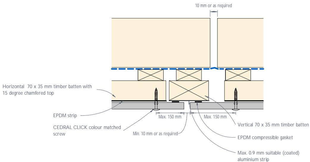
Figure 5: CEDRAL CLICK vertical control joint - Detail 2
