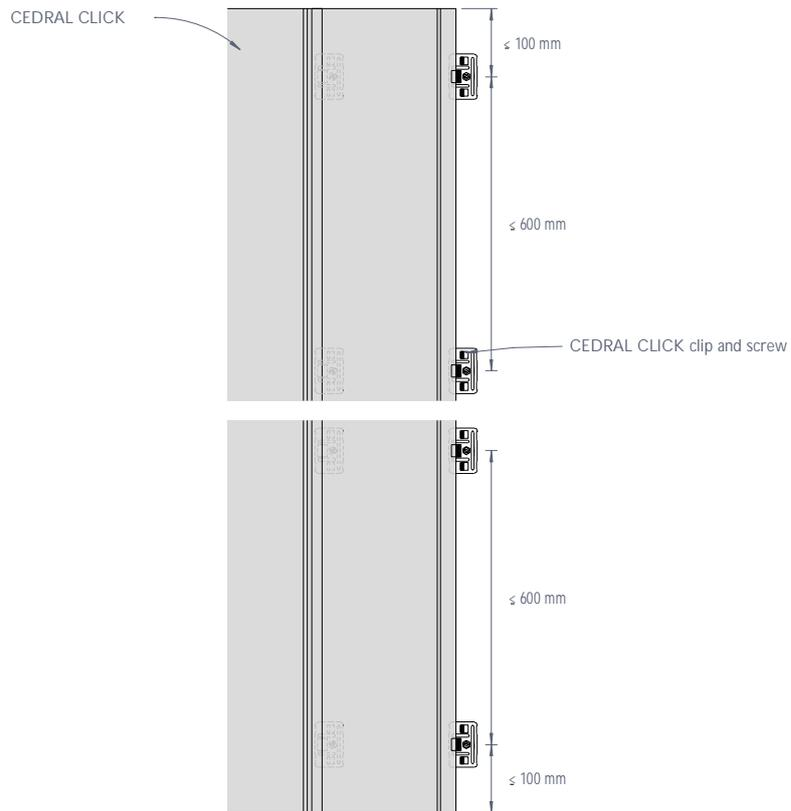
Figure 1: CEDRAL CLICK fixings arrangement - Elevation
