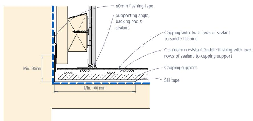
Figure 34: CEDRAL CLICK parapet junction - Section
