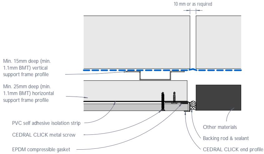
Figure 6: CEDRAL CLICK vertical control joint - Detail 3
