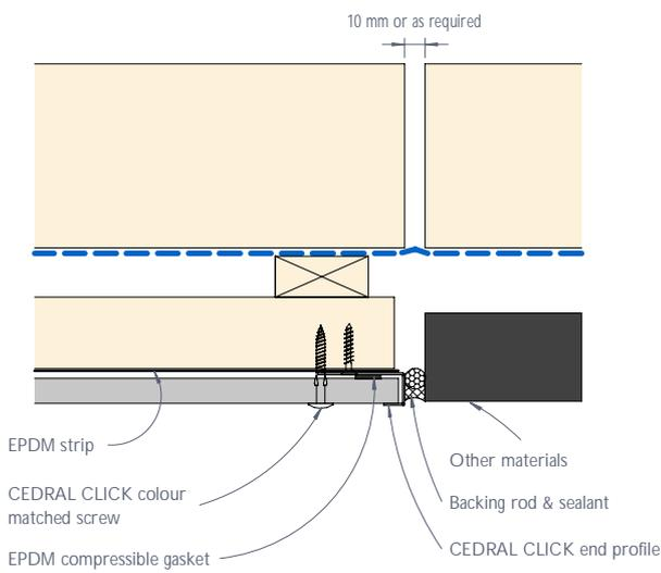
Figure 7: CEDRAL CLICK vertical control joint - Detail 4
