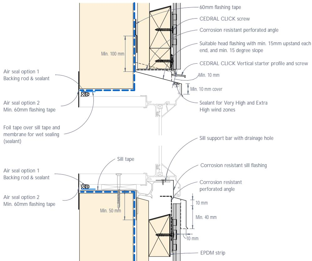
Figure 11: CEDRAL CLICK window head and sill junction - - Flush detail
