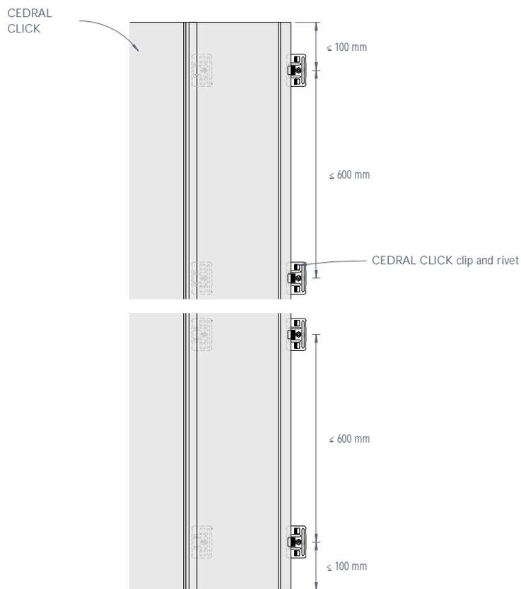
Figure 1: CEDRAL CLICK fixings arrangement - Elevation
