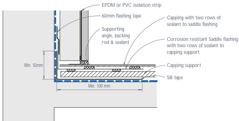
Figure 36: CEDRAL CLICK parapet junction - Section
