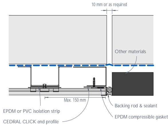
Figure 7: CEDRAL CLICK vertical control joint - Detail 3
