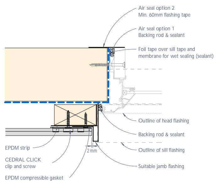
Figure 11: CEDRAL CLICK window jamb junction or the like Recessed detail option 2
