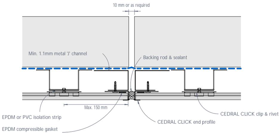
Figure 5: CEDRAL CLICK vertical control joint - Detail 1
