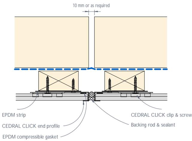
Figure 5: CEDRAL CLICK vertical control joint - Detail 1
