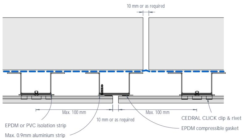
Figure 6: CEDRAL CLICK vertical control joint - Detail 2
