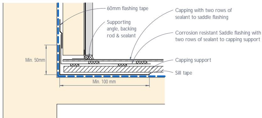
Figure 36: CEDRAL CLICK parapet junction - Section
