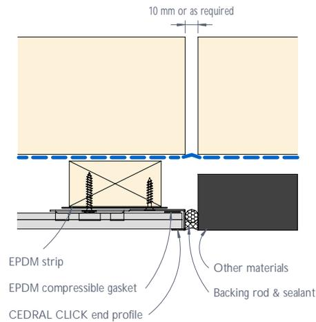
Figure 7: CEDRAL CLICK vertical control joint - Detail 3
