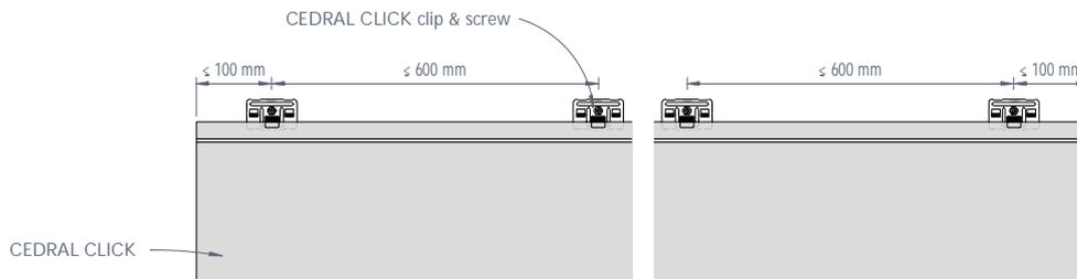
Figure 1: CEDRAL CLICK fixings arrangement - Elevation
