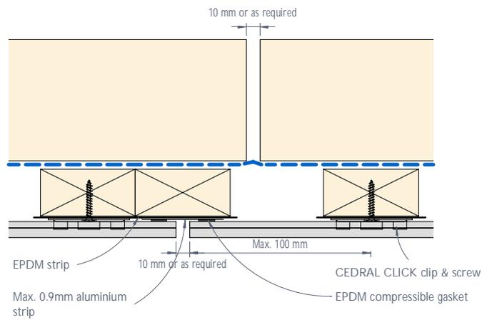
Figure 6: CEDRAL CLICK vertical control joint - Detail 2
