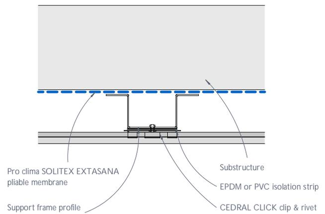
Figure 3: CEDRAL CLICK Intermediate fixing detail - Plan view
